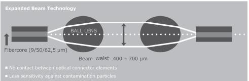
Expanded beam technology expands and collimates the optical signal through the connector interface path resulting in a diameter many times than the original beam. The optical beam is refocused into the core of the receiving fiber. This technology makes the connector very resistant to shock and environmental issues, minimizing the effects of dust and vibration. Because the lenses do not touch each other, the connector can be mated and demated for thousands of cycles.
