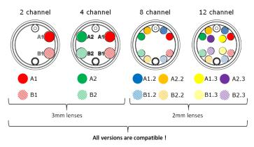
The EUROLENS system is the only expanded beam fiber optic connector system on the market where all 2 to 12 channel plugs and receptacles are fully compatible with each other.
